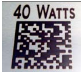
Figure 2: Black anneal marking using a combination of high repetition rate, pulse width control and a tailored mode.
