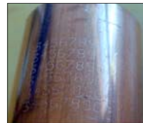
Figure 4: Engraving on copper tube with a 40 W HM (1.25 mJ, 20 kW, 30 kHz) and a 254 mm F-Theta lens: (top) 1m/s; (bottom) 6m/s
