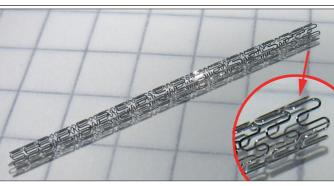
Using the fibre laser downtime has been halved, machine usability has jumped to well above 90% and the share of out of tolerance products has dropped significantly. On top of this comes the superior processing speed of the new system producing stents in just half the time the old plant needed. The overall result is a very substantial rise in the output of marketable products per unit and day.
